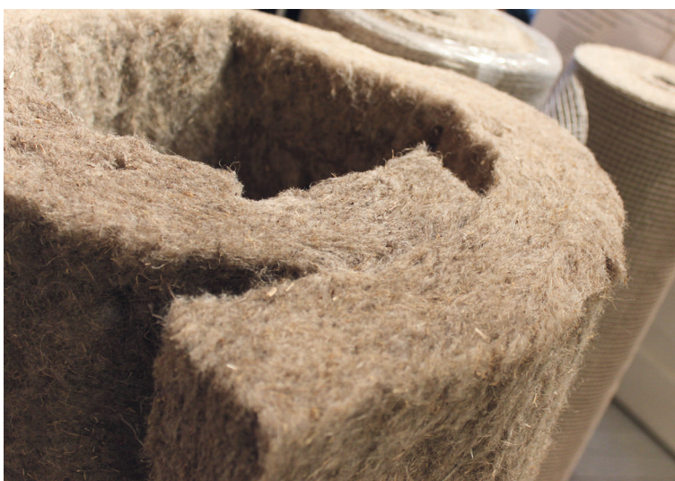
In recent years, several types of building insulation materials with low environmental impact have emerged. Insulation made of flax is one of those - a light, durable material with hygroscopic properties. Photo: Jonas Ulfsfält
