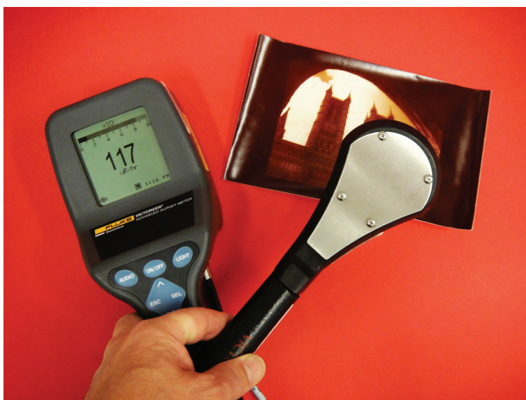
Figure 46 Noncontact radioactivity of a uranium-toned photograph is measured using a highly sensitive Victoreen Advanced Survey Meter.
