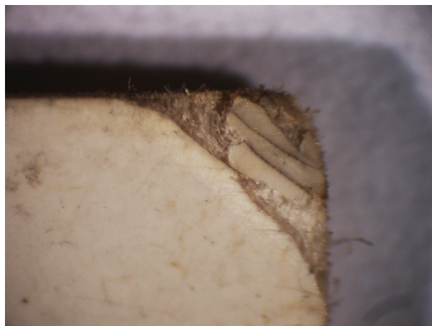
Figure 8b Detail of a POP photograph (40× magnification), showing the presence of the baryta layer at a damaged corner area.
