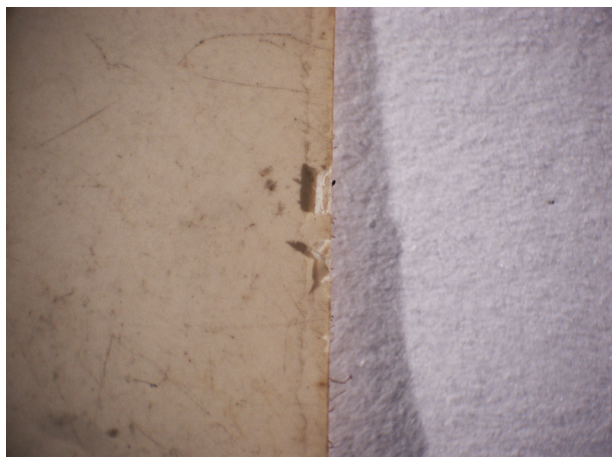
Figure 8a Detail of a POP photograph (40× magnification), showing the presence of the baryta layer at the edge area.
