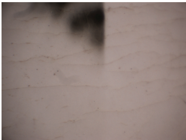
Figure 9 Detail of a typical pattern of mechanical damage to the surface of the gelatin layer (40× magnification).
