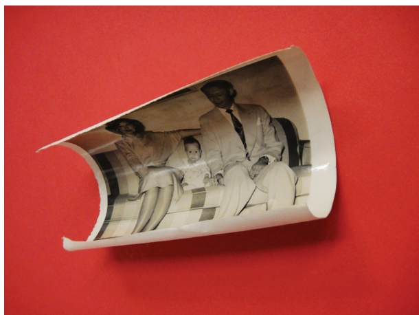
Figure 6 POP photograph showing a tendency to curl, which may indicate the presence of a surface coating.
