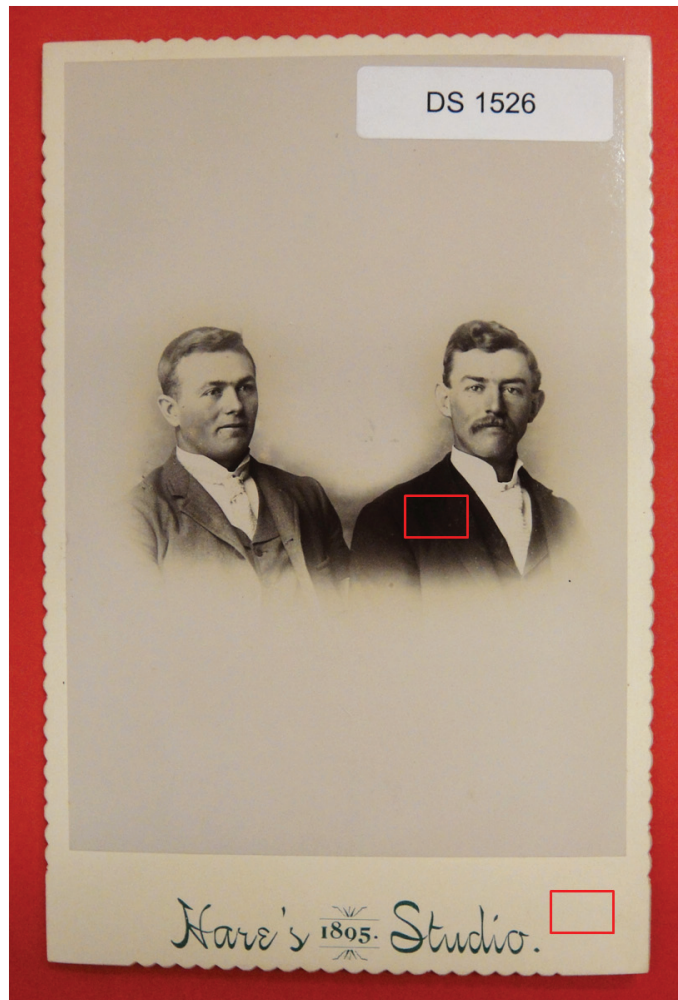
Figure 14a Cabinet card-mounted POP silver gelatin photograph indicating areas of XRF analysis.
